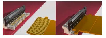
It is recommended to insert the flat cable in the correct pin direction.
