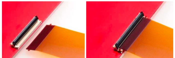
It is recommended to insert the flat cable to the zif connector avoiding bends/curves to safeguard good functionality.
